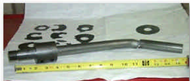
Figure 3-4. Broken tool arbor and cutting blades
