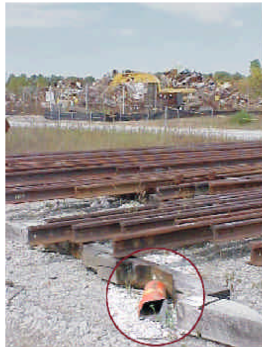
Figure 1-2. Portion of the fire extinguisher that became a projectile
