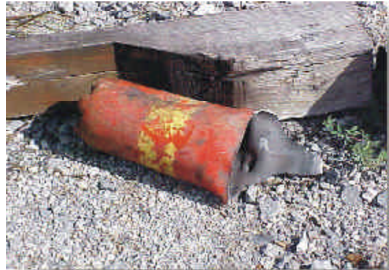
Figure 1-2. Portion of the fire extinguisher that became a projectile
